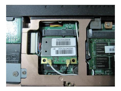
Step C, assign the Antennas (Aux. and Main) to the ipex connectors respectively,
